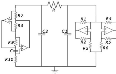
FIG. 6. Circuit diagram for the chua circuit used, except we used an inductor in place of the circuitry on the far left
