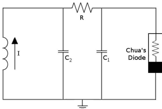
FIG. 1. Circuit diagram of a chua circuit
