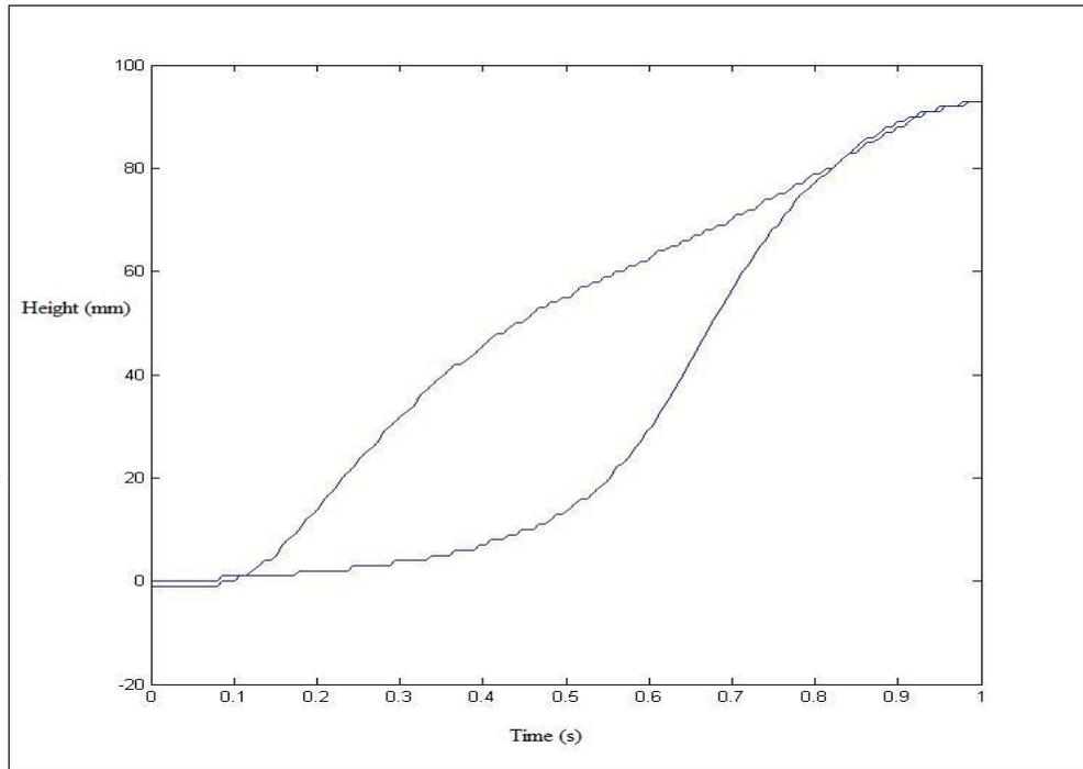
Figure 1: Height Hysteresis of Fluid during 1Hz Triangle Pulse
