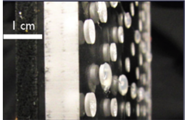
FIG. 5. Plexiglas magnet sheet with black sliding surface attached on the left.
