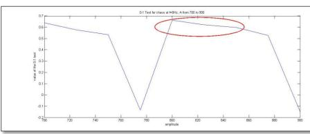
➤ Best results for f=7Hz and amplitude around 1100 counts and for f=8Hz between 800 and 875 counts.
