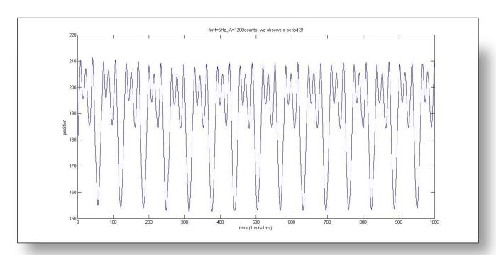
• High sensibility to initial conditions, for a fixed set (frequency, amplitude, initial position and speed), we observe two really different trajectories.
