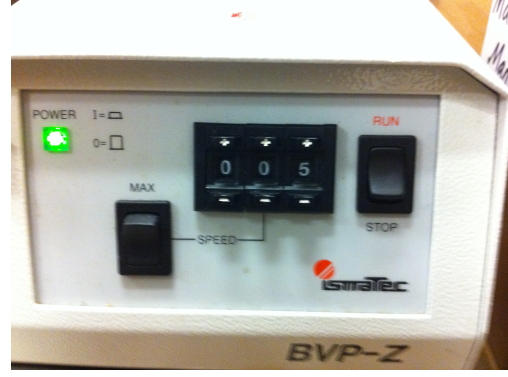
FIG. 5. Closeup of the Flow Regulator Control
