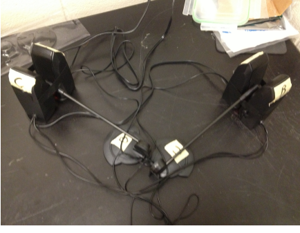
FIG. 2: This is the speaker/microphone couplings that modeled our crickets.
