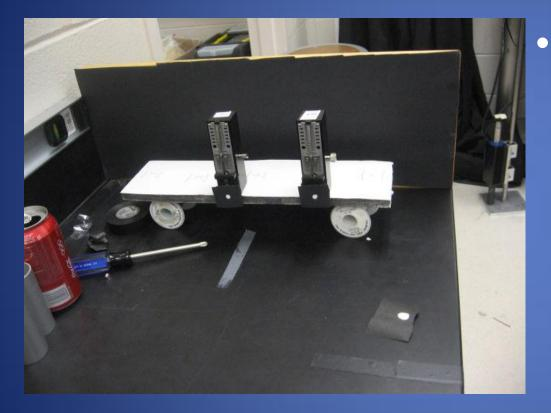
Metronomes were mounted on a foam board. This board rested on two rollers. Initially we used cans, but they proved unreliable so we switched to spools.
