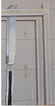
Figure 3: The final rig setup, with black tracking strip in place on the second arm of the pendulum. The first arm is taped white to reduce shadows and tracking artifacts.
